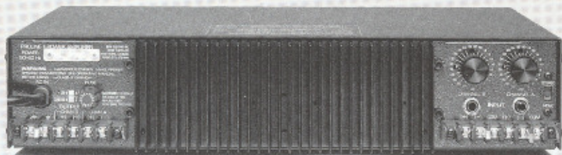
The Model 6500T rear panel includes barrier strips, phone jack inputs, gain controls, and mono bridging switch.
